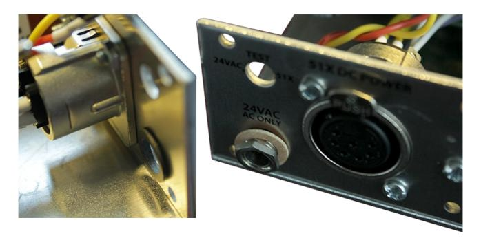
Using the round head screws & nuts, you will attach the 51X XLRs.
