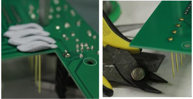
Later on we can cut to length by aligning with the MAIN PCB, to see where to cut.
