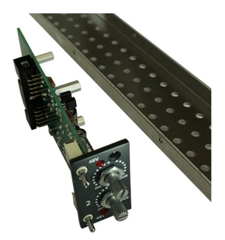
You will attach the Pots PCB to the side panel using the 3 fillister head screws and the pots panel using the 2 black phillips screws.
