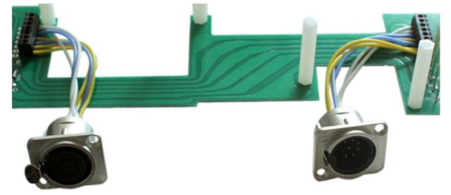
Also note: The 51X power-supply XLR input will normally be male to accept a female power cable XLR, but this will depend on how you wired your 51X power supply cable.
